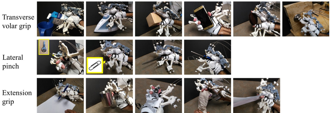
Fig. 4. A C5/C7 incomplete SCI subject, who is barely able to generate flexion of index and middle fingers, was able to grasp 15 objects listed in Sollerman hand function test. In the experiment, only four target hand poses of Maestro were used.
