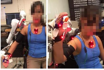
Fig. 2. Marker placement for the mocap system. Three markers were placed on the chest, used as reference frame, one marker on the right acromion process, one marker on the right olecranon, one marker on the right wrist strap, and two markers on the right hand palm. Since the hand attachment cuff restrains the wrist movement in all degrees-of-freedom, the set of markers consisting of the one in the wrist and the two in the palm have a constant geometric relationship, thus, they were used to obtain the hand frame.
